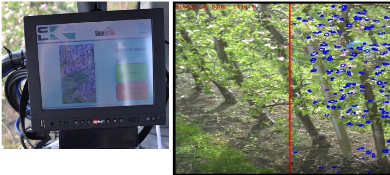
Figure 5: GUI (graphical user interface) of the camera system (left) and flower cluster recognized by the algorithm (CLK GmbH) (right).
