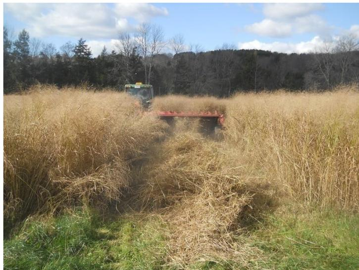
FIGURE 18. FAUCHEUSE ROTATIVE SANS CONDITIONNEUR
