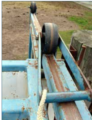
Figure 13. Rubber wheels on the rail
